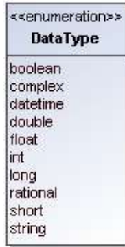
Figure 16: An enumeration is indicated by a box with the name of the the enumeration and the list of literals.
