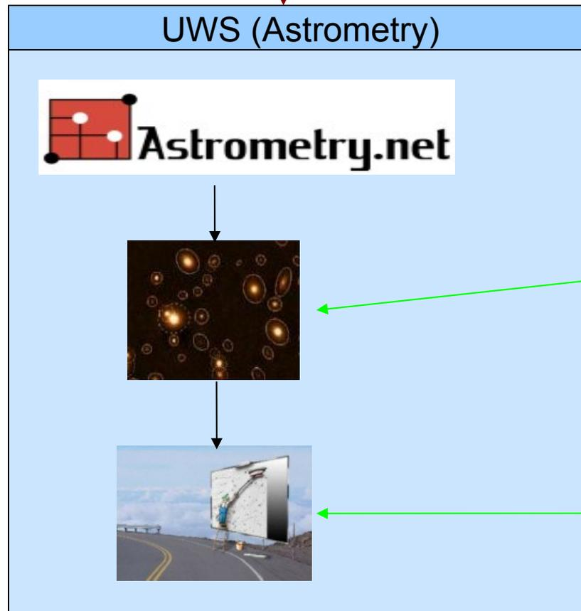
take the result of astrometry.net to compare source extraction (sextractor) with catalogues and make polynomial approximation of correction
