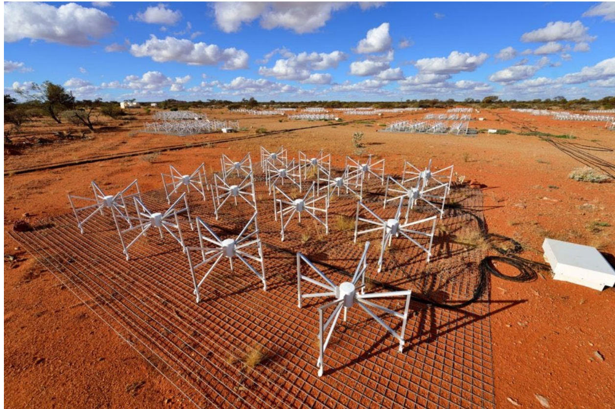
Foreground: One MWA tile has 16 dipole antennas and a beamformer (right)
