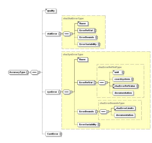
Figure 12: The accuracy element relies on Errors along the axes and is built up on STC elements.
