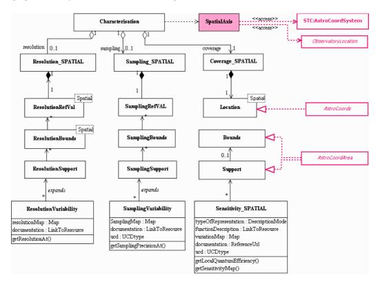
Figure 6: UML diagram: Expressing the spatial properties as a subtree of Characterisation. Here is an example of how STC components (in pink italics) may be used to implement the different levels of the Coverage description. The Location element uses a STC:AstroCoords. Bounds encapsulates STC basic types like STc:Interval elements and STC:Coords in a structure similar to STC:AstroCoordArea.
