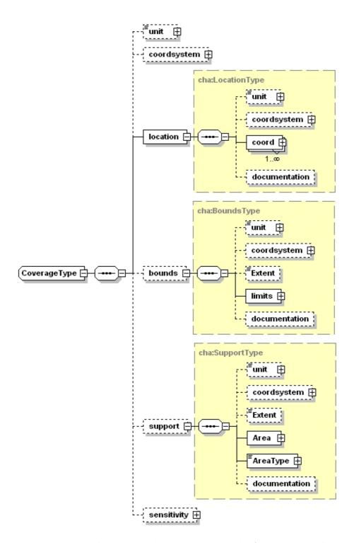
Figure 8: The coordsystem and unit items can be factorised at the top of the Coverage structure, but may be redefined at each level when necessary. **Bounds** are expressed using a limits element which is developed on a general bounding box type: CharCoordArea. AreaType is a string describing the kind of region used: Circle, Polygon etc.
