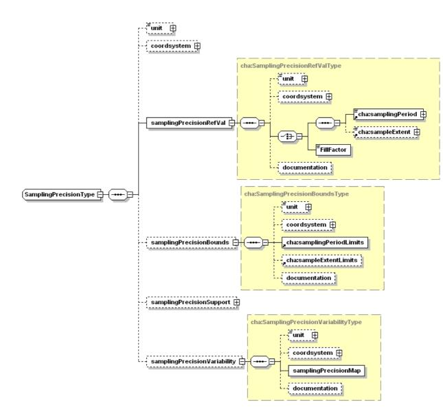
Figure 11: The samplingPrecision item contains 4 possible subelements. One among SamplingPrecisionRefVal and SamplingPrecisionBounds should be present when possible but this is not explicitly described by the XML syntax.
