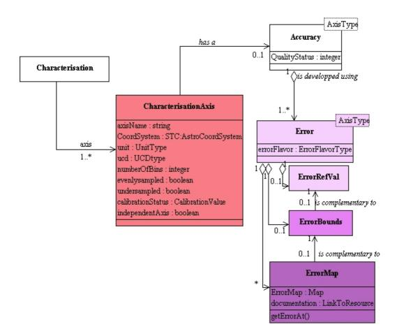
Figure 5: This class diagram illustrates the CharacterisationAxis class and its relationship with the Accuracy class, which encompasses various types of errors such as systematic or statistical.
